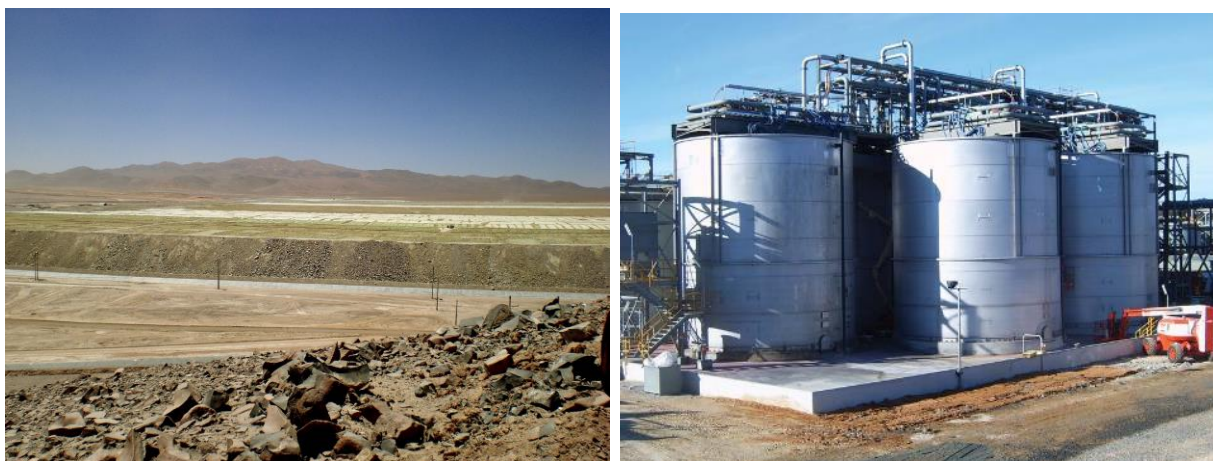
Left: biomining copper in by heap leaching; right: biooxidation of gold ore in stirred tanks
